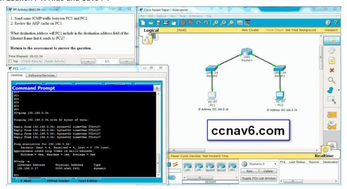
Open the PT Activity. Perform the tasks in the activity instruction and then answer the question. What destination address will PC1 include in the destination address field of the Ethernet frame that it sends to PC2?
